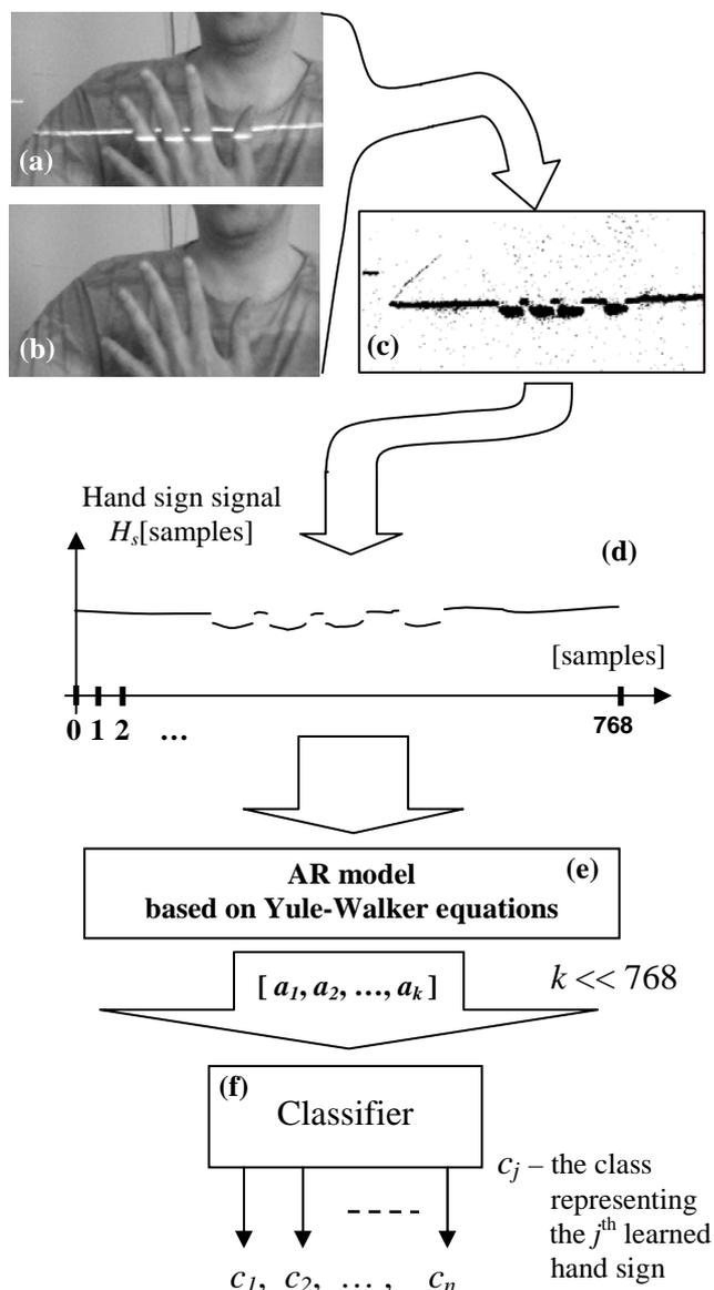
Figure 2. The system's flow chart
